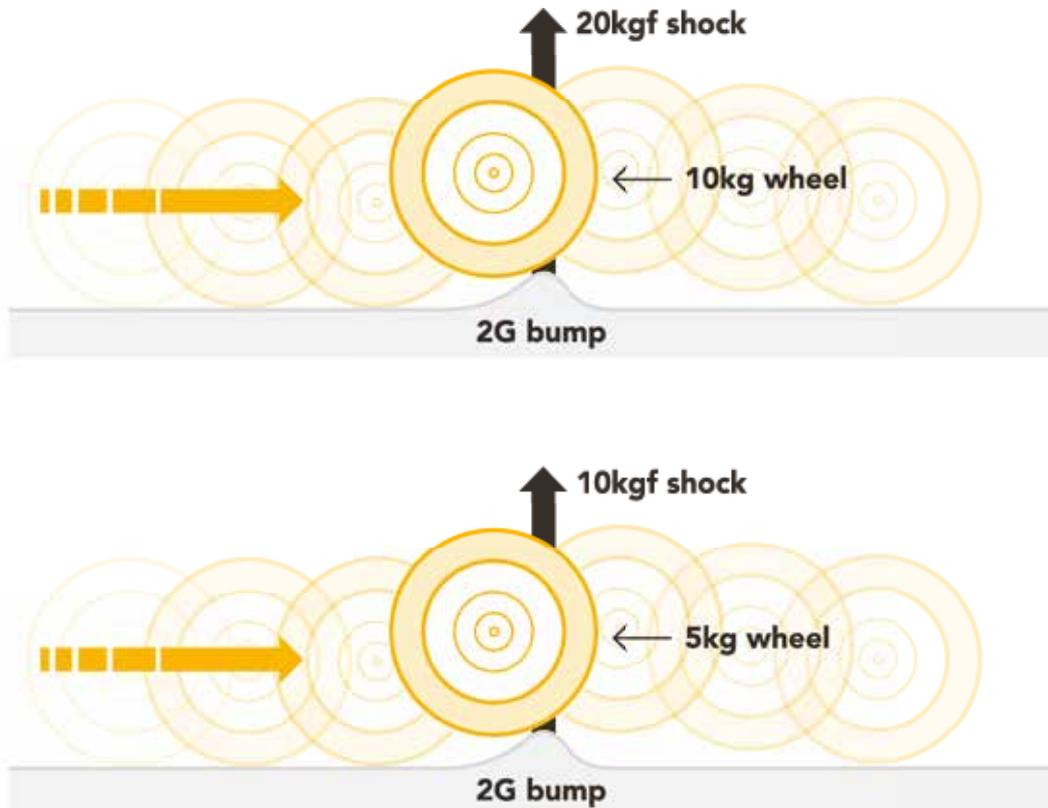
A high unsprung weight can also lead to “bouncing” and “hopping”, where the tyres temporarily lose contact with an uneven road, causing the bike to buck around – which is potentially dangerous.
