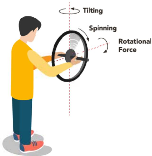
The equation for this rotational force is  $T = I\omega^2$  where the rotational force ( $T$ ) equals the wheel's MOI ( $I$ ) times the wheel's spinning speed ( $\omega$ ) times the speed with which you are trying to tilt the wheel ( $\theta$ ). Importantly, the rotational force with which the wheel resists your tilting depends on the MOI. *A wheel with a low MOI will therefore exert a lower rotational force as you try to tilt it.*
