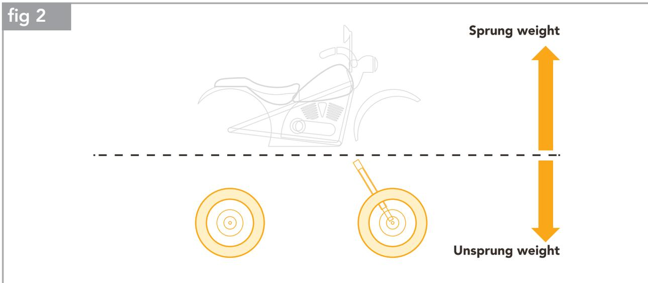
When a bike passes over a bump in the road, the rider will feel the unsprung weight being forced upwards. At high speeds this causes unpleasant vibrations - the greater the bike's unsprung weight, the stronger these vibrations become.:
